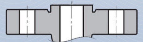
TYPE G AND H - O-RING SPIGOT AND O- GROOVE FACE
