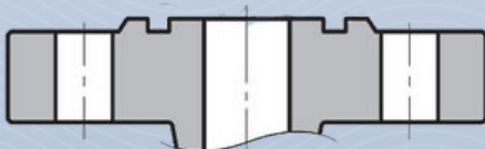
TYPE C AND D - TONGUE AND GROOVE FACE
